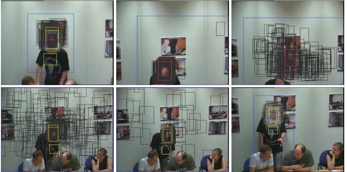
Fig. 14. Lost and found - functionality of the particle filter. Frames of TS1 for t = 1309, 1324, 1337, 1383, 1384, and 1403 are displayed. (The additional partitionings in the top of the upper rectangles in this and the following figures belong to a third object profile not reported in this article.)
