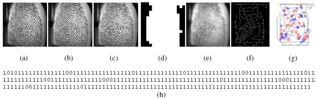
Fig. 9: (a) Input Fingerprint Image (b) Histogram Equalized Image (c) Median Filtered Image (d) Segmented Image (e) Enhanced Image (f) Morphological Processed Image (g) Fingerprint images with Minutiae Points (h) Generated irrevocable key.
