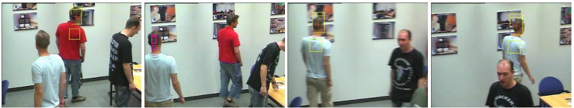
Fig. 20. Interactive selection of another target object. The frames t = 1815, 1845, 1870, and 1923 of TS3 are displayed. In the second image the man with the white T-shirt is selected for tracking instead of the previously tracked man with the red T-shirt. He is successfully taken over by the tracking module.
