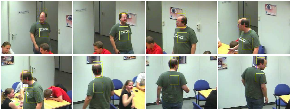
Fig. 15. Exposure to changes in camera parameters - pan. Depicted are frames t = 475, 500, 545, 580, 615, 655, 675, and 700 of TS2 which render snapshots of a smoothly panning camera. Two competing reference profiles used as described in subsection II-H are crucial for the successful tracking of this sequence. The proposed system can keep track with the camera movement.
